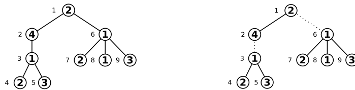
■ Figure 1 Left: A weighted tree t . The small numbers next to the nodes denote their IDs. The trace of a depth-first-traversal of t is 2412\bar{2}3\bar{3}1412\bar{2}1\bar{1}331\bar{2} , where we ambiguously write w for (‘d’, w ) and \bar{w} for (‘u’, w ). Right: Partitioning of t into three parts with bottleneck value 7. A streaming algorithm should output the IDs of the root nodes of the created partitions. Here, these are 1, 3, 6.
